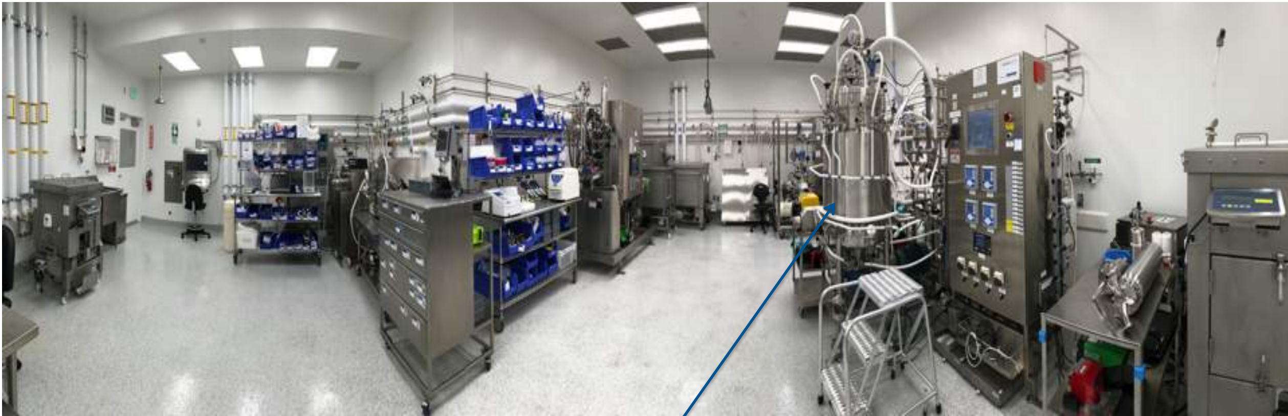
Continuous culture (chemostat) bioreactor for the cell-free extract (XtractCF™) production
